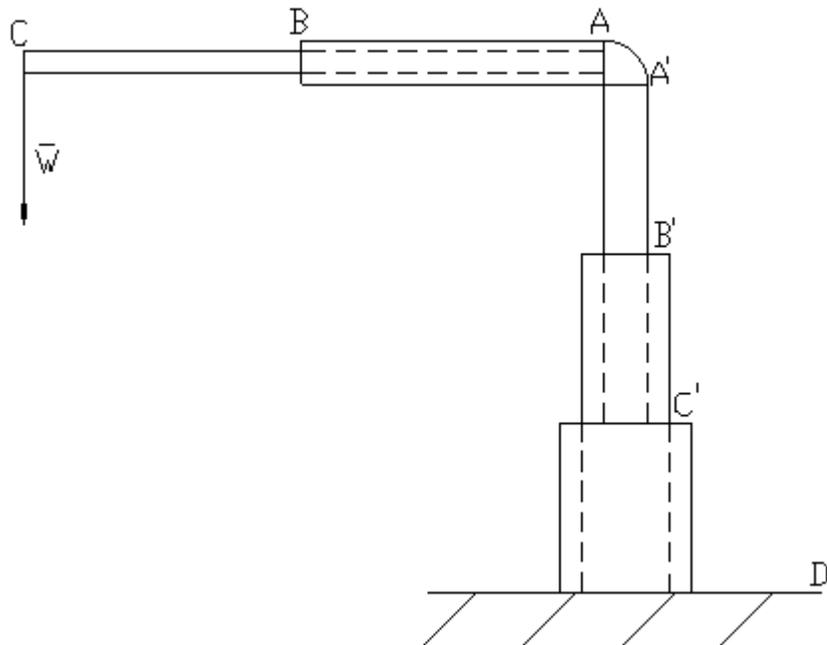
The crane will need both the vertical and the horizontal elements telescopic, in order to reach the required configurations when operative and to reduce its dimensions to acceptable ranges when off. This
