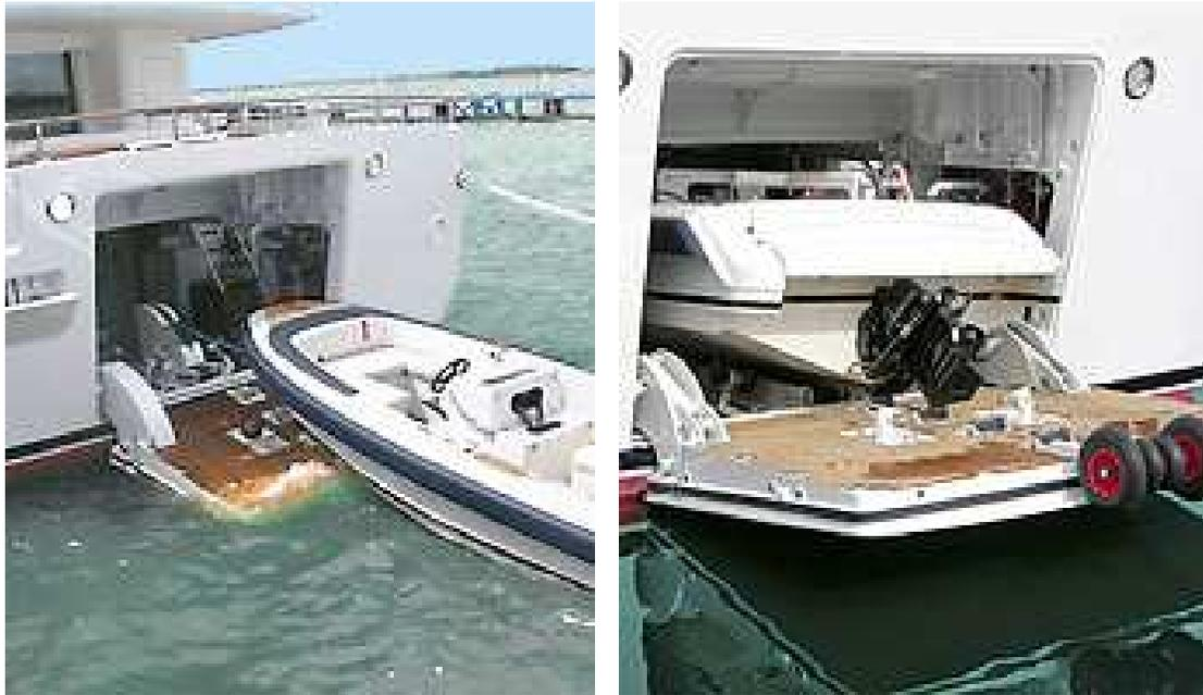
The vessel shown in fig. 4 is a brilliant example of this. Dutch manufacture, 33m yacht *Bystander* features a launching device for its tender which is aided by just thin flexible elements and wires, proper 'fishing rods' that guarantee a simple design, a cheap implementation and a very low weight together with an easy handling once the tool itself is operative.
